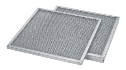
**Application:** The **HI SERIES INDUSTRIAL GRADE FILTER** is designed for use in residential, commercial and industrial HVAC applications to remove airborne particulate and coolant mist from the airstream. It can be used dry or coated with Filter Coat and is built to withstand repeated cleanings. Select from three different metal alloys to obtain the best filter for your application.
